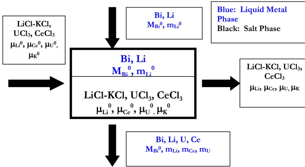
**Figure III.2:** Simple Molten-Salt/Liquid Metal Extraction System. Here Li is the reductant and the actinide chloride is the oxidant.
