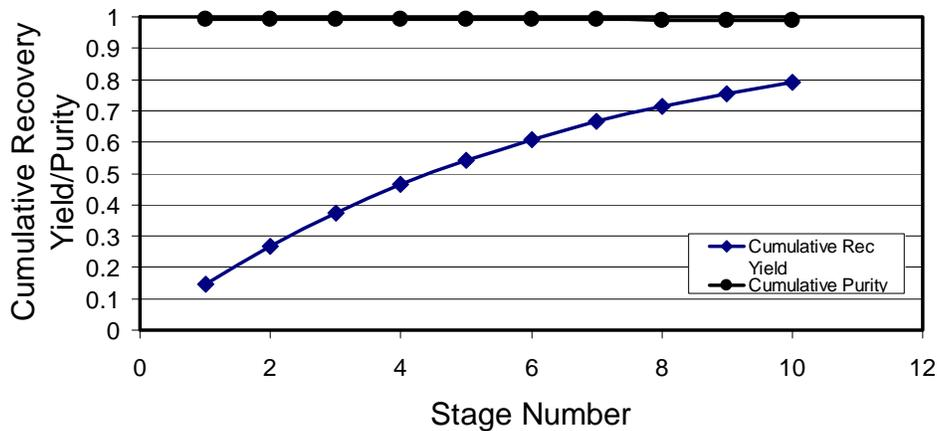
**Figure III.8:** Cumulative Purity and Recovery Yield as a function of stage number. Note the steady increase in recovery but slight decrease in purity.
