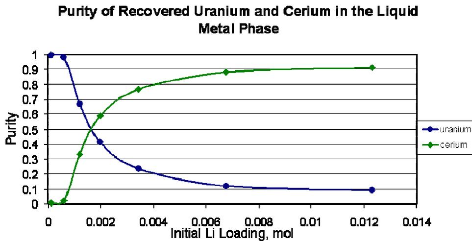
**Figure III.6:** Purity of U and Ce as a Function of Initial Lithium Loading
