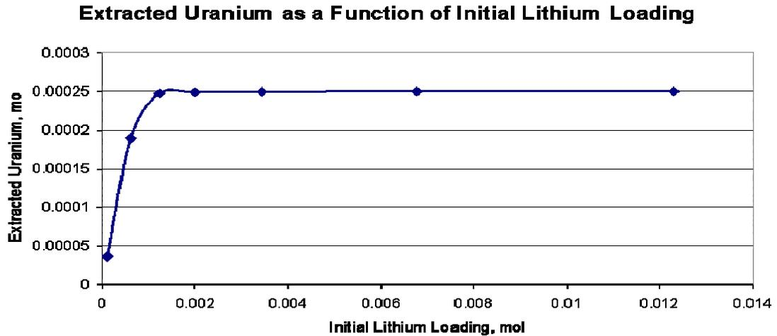
Figure III.4: Extracted Uranium as a Function of Initial Lithium loading.
