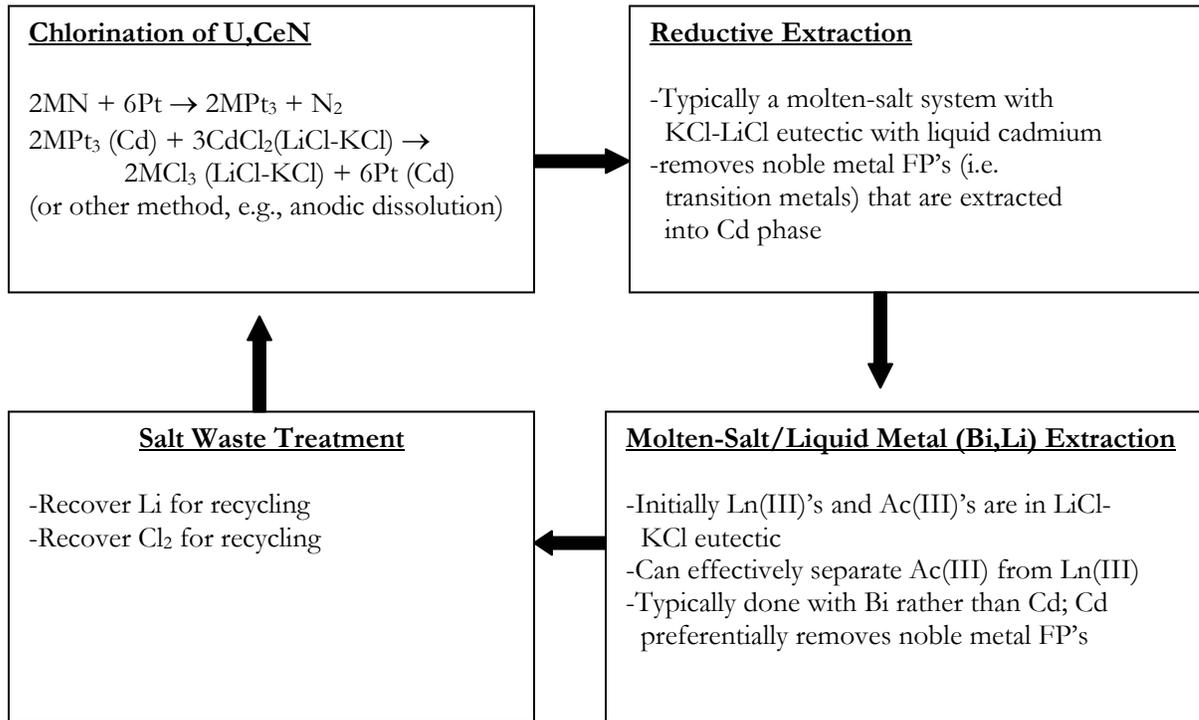
**Figure III.1:** A pyrochemical treatment of uranium mononitride<sup>3</sup>.
